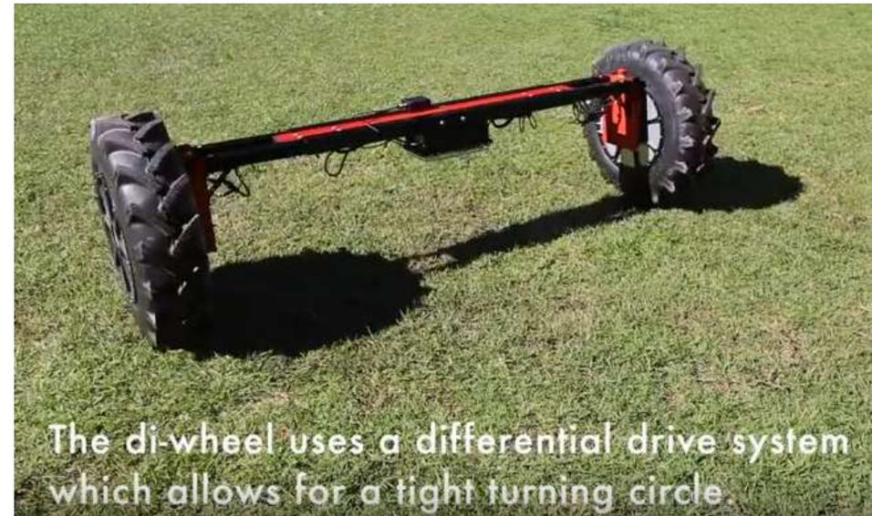
The di-wheel uses a differential drive system which allows for a tight turning circle.
